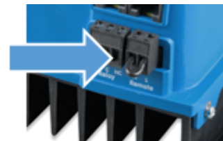
Remote connector with the wire loop.
