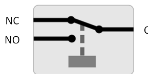
Relay configuration (not energised).
