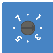
Rotary switch set to position 2
