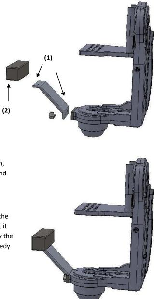
this by adjusting the camera platform up or down so the camera's center of mass is on the center of tilt rotation.
