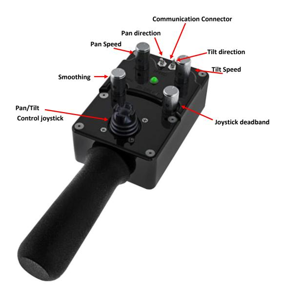
**Communication connector (Green)**- Connect this to the communication cable, and connect the other end of the communication cable to the green connector on the CinemaPro Head. This cable runs communication as well as power, so make sure that there is XLR power connected to the CinemaPro
