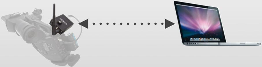
Cube Encoder *creates* the network, the computer *joins* Cube's network. VLC on the computer *decodes* the video for playback.
