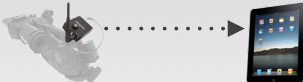
When streaming to an iOS device, the same ad hoc and infrastructure network configuration rules apply. This example shows Encoder to iPad Ad Hoc.
