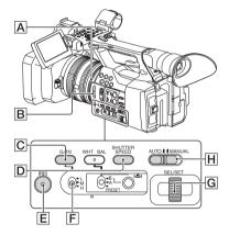
You can adjust the image brightness by adjusting the iris, gain or shutter speed, or by reducing the light volume with the ND FILTER switch  $\blacksquare$ .
