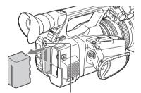
BATT RELEASE (battery release) button
