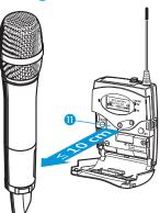
The parameters are transferred to the transmitter. When the transfer is completed, " $\checkmark$ " appears on the display panel of the diversity receiver. The receiver then switches back to the current standard display.
