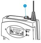
The ground connection of the line cable serves as the antenna for the second diversity section. For details on the connector assignment, refer to the diagram on page 24.
