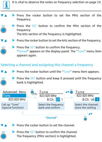
Set the desired frequency (MHz and kHz section) as described in the previous chapter.
