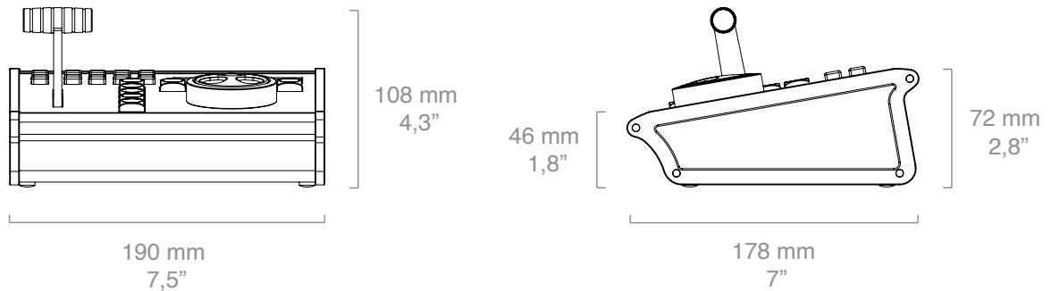
Figure 1: Technical drawing of Time Spin with key dimensions and layout details.
