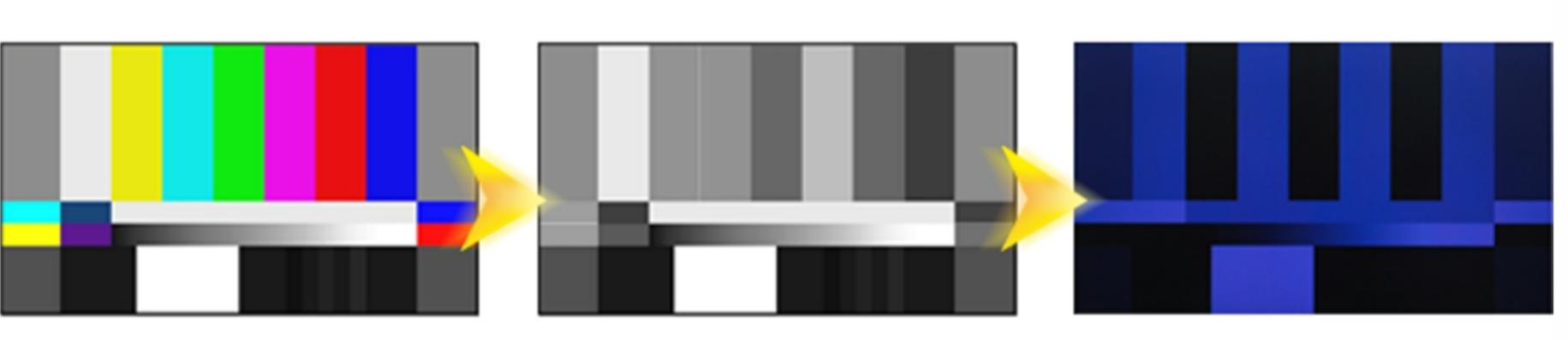
the Blue only image can check and adjust the monitor saturation based on the SMPTE testing signal, which is one of the necessary and important methods those use for field debugging the monitor
