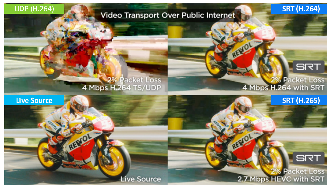
Picture quality comparison at 2% packet loss (UDP vs SRT)
