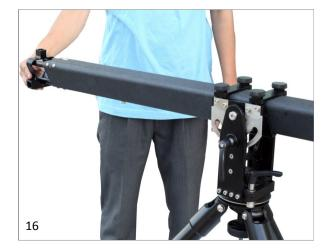
Now attach Section-3 with Section-2 and Section-4 with 3<sup>rd</sup>. Insert the other clamp into Section-4. Repeat this process for rest of the sections.
