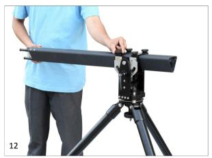
• Lock both the pan and tilt knobs to assemble the Jib crane.
