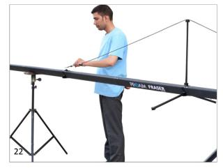
• Similarly, attach 18.5ft long (Red) cable from Section-1 to the end of Section-7, while aligning it with Cable Guide Top Rod.
