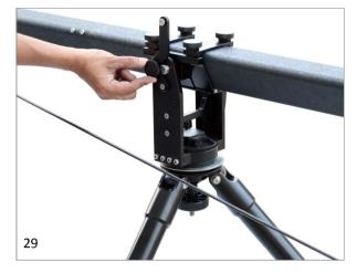
• Similarly, loosen the knob on Head Plate, slide it inside to pull a small part out of it, for fixing cable later. Tighten the knob properly to secure it.
