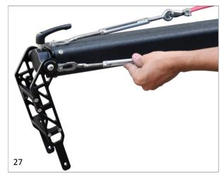
• Loosen side knob of Hub Mounting, slide it upwards to pull a small part out of it, for fixing cable later. Tighten the knob properly to secure it.
