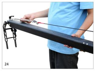
• Now connect both 18.6ft long (Blue) cables on each side of Section-1.
