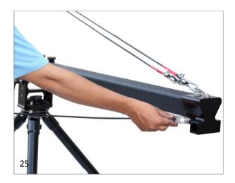
• Align both the (Blue) cables with Cable Guide Side Rods and further fix them at the end of Section-7.
