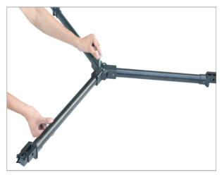
• Pull out the locking pin from the wheel in order to attach it to dolly. Repeat this process for all the wheels.
