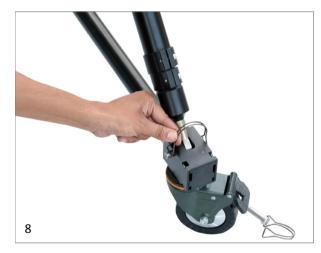
• Place the Hub Mounting on Jib Stand and tighten it with the hub locking knob to secure it.
