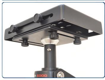
The camera platform:- moves back and forth, and side to side, to quickly allow you to adjust the cameras horizontal balance. By varying the amount of counterweight disks on the base platform you adjust the camera's vertical balance. When balanced properly the camera floats, ready for you to move into action.
