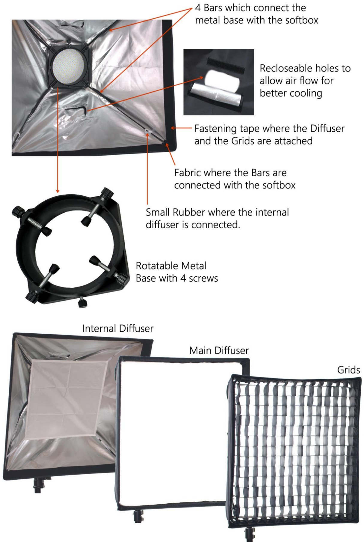
DIAGRAM 14 (Softbox assembling)
