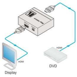
Figure 2: Connecting the PT-1C EDID Processor
