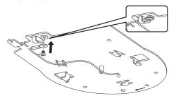
2 Place the supplied template against the ceiling, and fasten the ceiling mount bracket with four screws (M4 wooden screws: Φ4.1).
