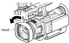
To attach a hood, press it against the lens, and turn it in the clockwise direction.
