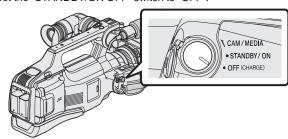
2 Remove the power source (battery and AC adapter), connect these again, and then turn on the power. (Reset completed)
