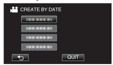
If the desired date cannot be found, switch the mode to video (60i), video (60p), or still image accordingly in step 2.
