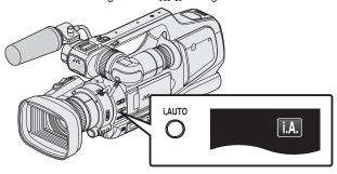
• If Manual (M) is activated, switch to Intelligent Auto (i.A.). "Selecting Intelligent Auto/Manual Recording Mode" (☞ p. 18)
