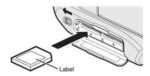
• Insert with the label facing upwards.
