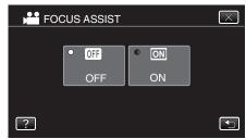
The screen is displayed in black and white, and contour of focused parts are highlighted in color.
