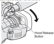
To attach a hood, press it against the lens, and turn it in the clockwise direction.
