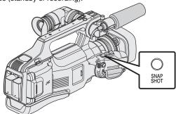
• "PHOTO" lights up on the screen when a still image is being captured.
