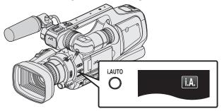
• If Manual (M) is activated, switch to Intelligent Auto (i.A.). "Selecting Intelligent Auto/Manual Recording Mode" (☞ p. 18)
