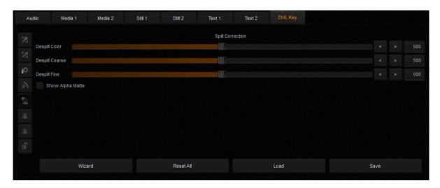
**Despill color** and **Despill coarse** belong to the functions for the preliminary elimination of unwanted colours, and are based on the RGB space.
