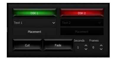
To configure position and size of the downstream key, click on the placement button to open the window shown below.
