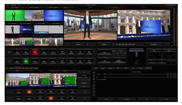
Once the virtualset is imported into the production live module, you can preview your virtualset in the PVW screen. Configure your virtual studio in the Virtual Studio Configuration Panel. Each phase corresponds to a virutal camera position. The user can switch between phases by clicking on phase windows, which is similar to the "cut transition" effect on a switcher.
