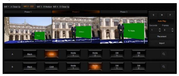
The virtual studio configuration panel is located at the bottom left-hand corner of the screen. Two rows of buttons located below the three phase windows serve the purpose of allowing the user to select talent material source and green screen material source. As depicted in the diagram above, row A is for talent material source selection and row B is for green screen material source selection.
