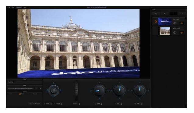
After all graphic layers are arranged in place, import the screen layer (Source B), which will be shown in VIRTURALSET maker as a green rectangular box.
