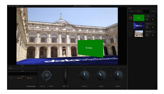
Please note that the Virtualset Maker allows the user to place up to **six screens** on the studio layer. Once all six layers are selected, Source B option will then no longer be visible in the "**Select layer type**" dialogue box.
