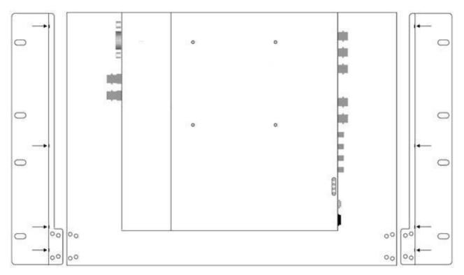
Use the supplied screws to attach the left and right rack ears. You will there are four screws either side, as illustrated above, plus additional screws at the base of each rack ear, as illustrated below.
