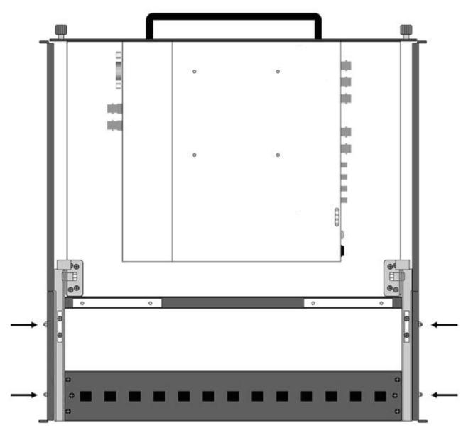
Mount the monitor in your rack with the rear panel facing upwards. Ensure the rack mounting screws are secured both front and rear.
