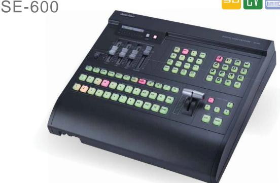
The Datavideo SE-600 is an eight input Standard Definition video switcher, with built in dual channel audio mixer. The SE-600 provides 6x Composite Video, 1x DVI-D and 1x DVI-I input with Multi-View output displaying each input, as well as Program & Preview on one monitor.
