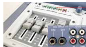
Built in audio mixer with 2 microphone channels, 1 aux video source input
