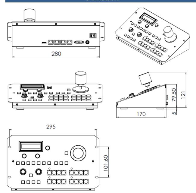
All measurements in millimeters (mm)
