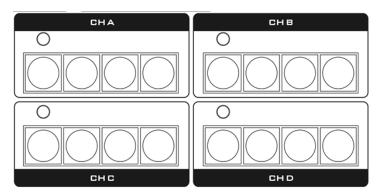
5. The selected preset button will remain ON for 2-3 seconds and the button LED will be turned OFF after the settings are successfully saved.
