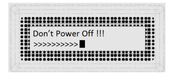
9. After the bootloader is upgraded, the LCD panel will show the following and the user may proceed to upgrading the application firmware.
