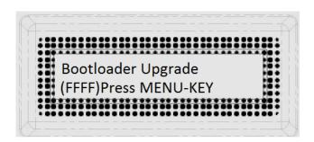
8. Press the MENU key to start the bootloader upgrade and do not disconnect the power before the upgrade is complete.
