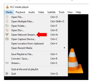
On the window that opens, enter rtsp://IP address:554/channel number as shown in the diagram below then click Play to start viewing.
