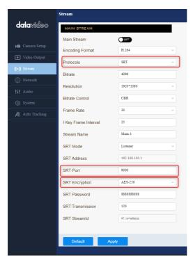
Caller and listener modes work together to establish the SRT link between source and destination devices. It is arbitrary to set one device to listener mode and the other to caller mode. Either can be the source device.
