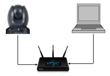
After connection has been successfully established, on your PC/laptop, use DVIP Configuration Tool to search for the camera's IP address. If you are new to DVIP, see the <u>DVIP</u> section for more descriptions of the tool.
