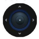
Use the up/down arrows to tilt the camera head up and down and the left/right arrows to pan the camera head left and right. You can also use your mouse to drag the central dot to control the camera's up, down, left, and right movements.
