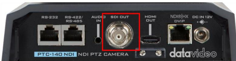
Connect the SDI OUT to an external connected monitor using an SDI cable.
