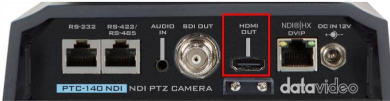
Connect the HDMI OUT to an external connected monitor using an HDMI cable.
