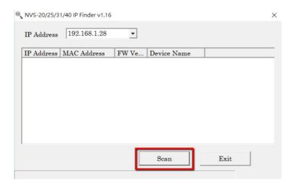
Step. 11. After the connected NVS-40 IP address is shown, please enter the IP address into the address bar of the web browser.
