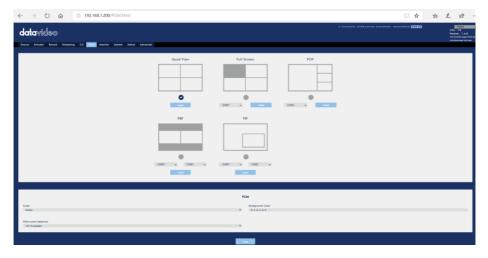
1. Quad View: Please press the "Quad View" icon and then please press the "Apply" button for applying the setting.
