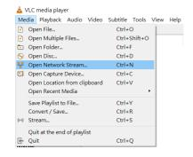
13. Please enter the streaming address that is generated by the NVS-40 into the "Please enter a network URL" column and then please press the Play button for playing the streaming. Take above address as an example, the address will be udp://192.168.100.100:1000
