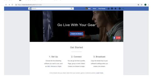
5. The following screen will be shown, please check "Use a persistent stream key" and then please copy "Server URL" and "Persistent Stream Key". Finally, please paste them into the "RTMP URL" column and "Stream Name" column respectively in the Streaming option of the NVS-40 web-based control interface.
