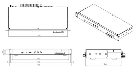
All measurements in millimeters (mm)
