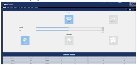
For the input source, if "Line-in" or "XLR" is selected, there is a slider for users to adjust the volume. However, this interface also allow users to select the audio source to be "SMPTE", "EBU" or "Manual". After the setting is finished, please press the "Apply" button to apply the setting.
