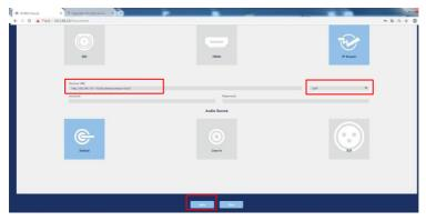
The input source related information will be shown on the bottom of the "Source" page. If the streaming video is decoded by the NVS-40 correctly, the word "IP Stream" and resolution will be shown.
