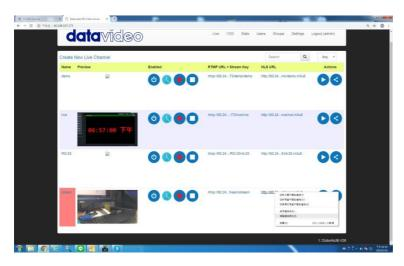
Step 2. Please click "IP Stream" from the web UI of the NVS-40 and then please paste the copied streaming address to the "Source URL" column in the IP Stream interface. After that, please press the "Apply" button. Note: If there is no special need, please set this "Source URL" column as UDP.
