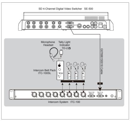
The ITC-100 is an ideal accessory for the Datavideo SE-2000 Video Mixer. The SE-2000 has four channels, each channel can connect to the ITC-100SL.
