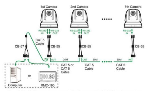
[Remark] The CB-57 cannot be connected with a Computer and a RMC-190 at the same time.
