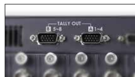
Advanced tally feature for easy connection to external systems such as Datavideo ITC-100 or TB-5
