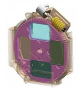
A compact, independent internal 3-density ND filter allows optimum exposure in various lighting environments.
