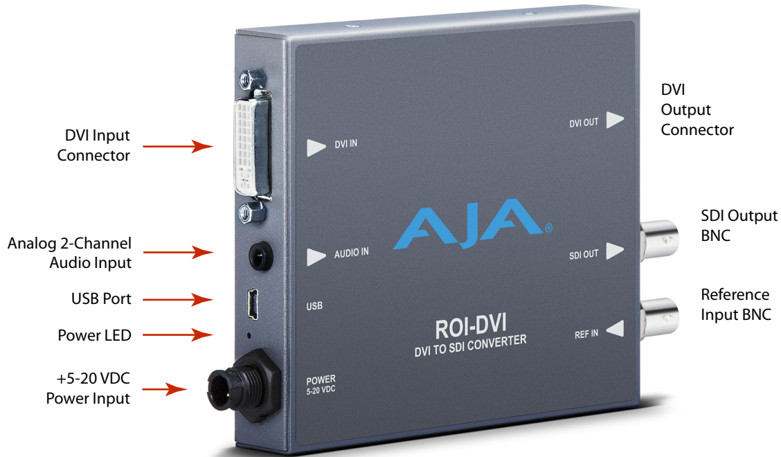
Figure 4. ROI-DVI Converter/Scaler
