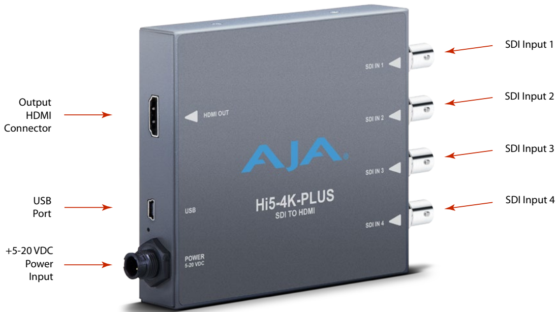
Figure 2. Hi5-4K-Plus Converter Connections
