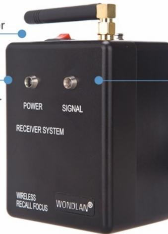
Signal display lamp, it twinkles when receive signal from controller
