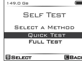
The User can choose between quick test and full test. Choose quick test. Quick test uses S.M.A.R.T test offered by the hard drive
