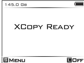
After checking the system, the NVSPRO goes into [XCopy ready] mode. You can copy a memory card in this mode.
