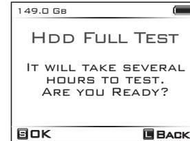
Full test takes several hours. The full test tries to read all the sectors in the internal hard drive and find out if any bad sector exists or not.
