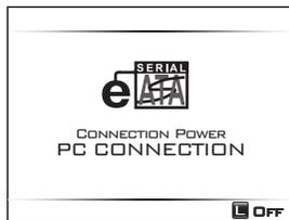
The eSATA cable does not provide power. Use the AC power adapter unit or USB/Firewire cable to provide power. If no power is provided, the NVSPRO shows the "Connect power" message and waits for external power to be applied.
