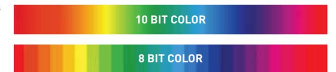
Even if we receive 8-Bit video as a source, we always record 10-Bit depth, to make combining high bit rate computer graphics and animations easier in post production.
