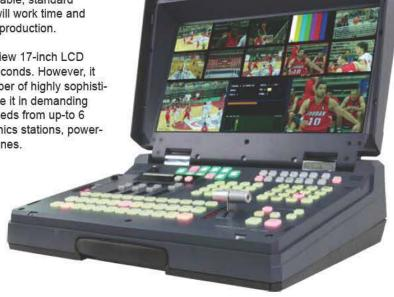
The complete system includes a single, secure power supply from one connection. Where the production is taking place away from the studio and mains power is unavailable, the HS-600 can even be powered from a 12v DC car battery.
